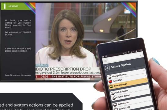
Each display device in the Intevi IDT system can be uniquely controlled and system actions can be applied across a group of screens. Branded templates can be displayed in two modes with full or minimal branding. The system operator can centrally control channel selection, apply different templates or send full screen alerts or display on screen messages on individual, groups or all screens.
