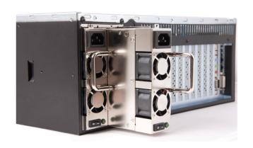
The PIPView BlackBIRD range of video wall processors offers new levels of performance and flexibility whenever you need multiple screens for command and control, showcase, collaboration or in retail. Using cutting edge technology for the capture of live video feeds, processing into easily defined layouts and finally output to up to 64 screens each showing full 1080p resolution.
