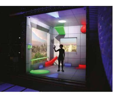
The application is a six-wall structure with 3D stere-oscopic projection displayed on all the walls / screens by 12 projectors. The image is generated on all screens and has the unique perspective shown to the user equipped with leading glasses. The Laboratory is now used as application helping to determine the future use of virtual Reality in other fields of science and industry. It is also an excellent basis for research and development of VR Technology (Virtual Reality).
